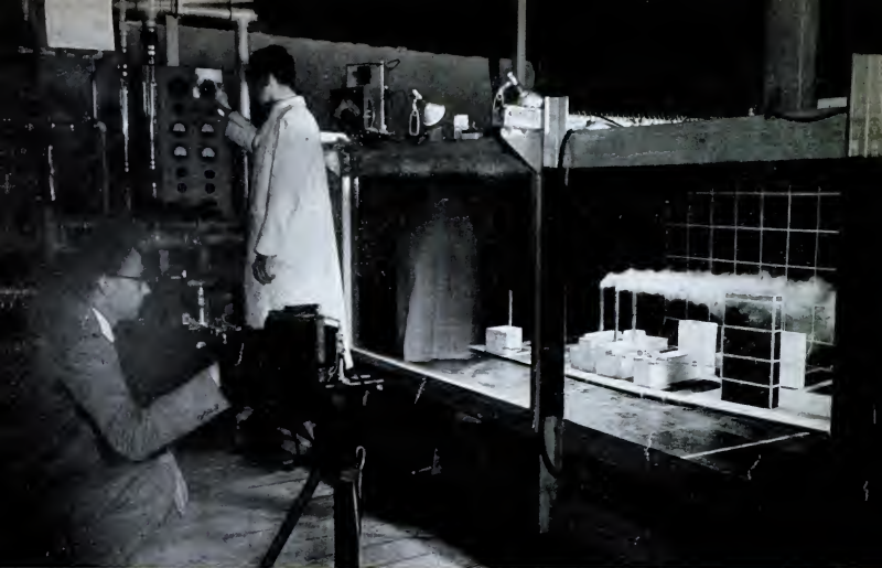
The smoke tunnel in operation. Models above show how the Waterside plant shrouds the
